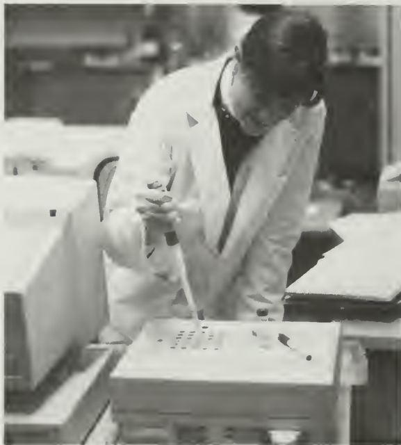
FIGURE 5-3: HWRIC QA SPECIALIST CONDUCTING MICROTOX TESTING ON WASTEWATER SAMPLES
